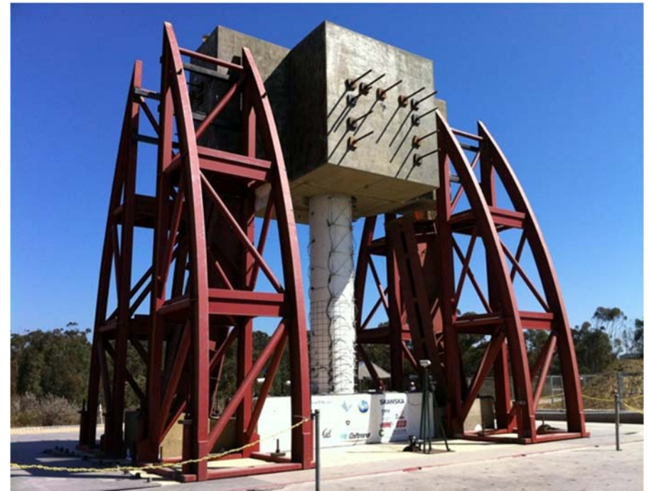
Full-scale 1D tests of circular column - Jose Restrepo, PI (PEER, Caltrans, UNR, FHWA, NEES@UCSD, NEEScomm & NSF)
